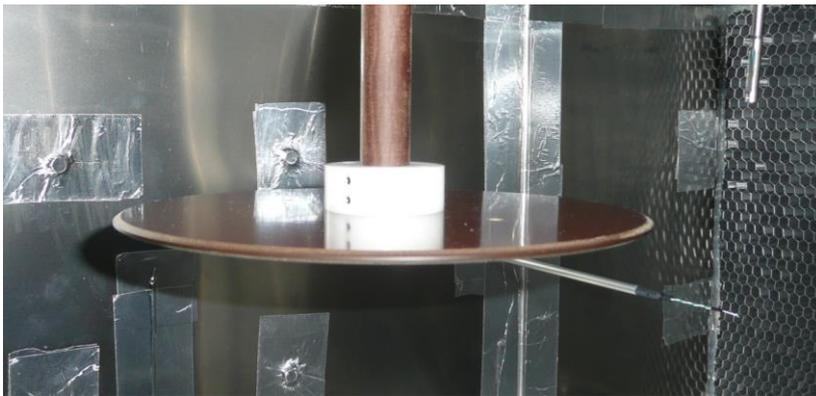
Rotating detector mount in tunnel next to temperature and airspeed sensors
